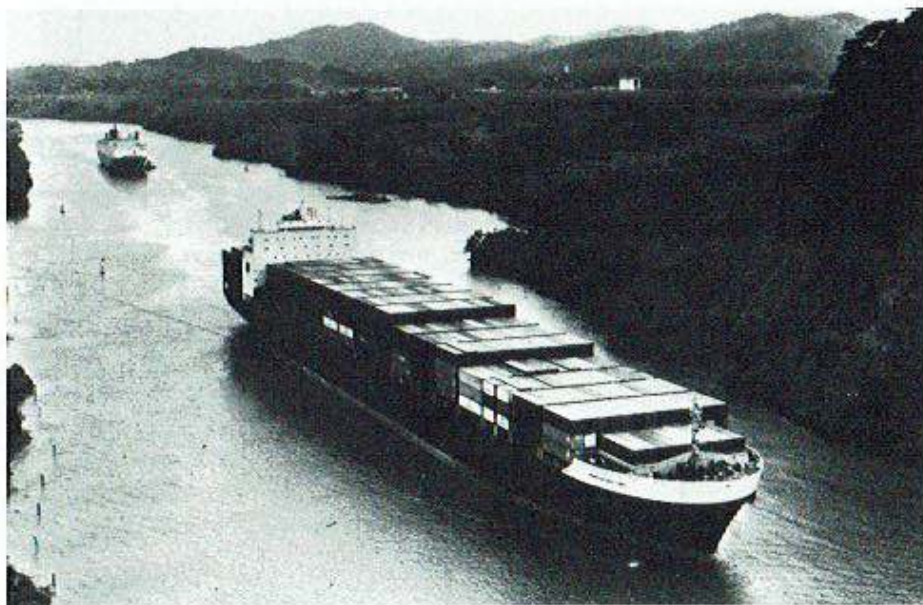
One of McLean's Jumbo Econships, The M.V. AMERICAN NEW YORK, on her maiden voyage, transiting the Panama Canal. This vessel and her 11 sisters were, in 1984, the world's largest containerships, with a capacity of 4456 TEU. (These vessels are now Sea-Land's Atlantic Class)
