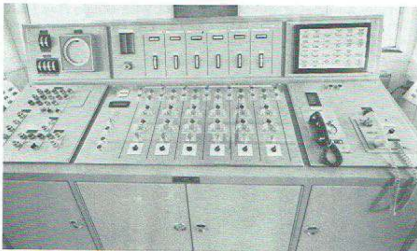
FIGURE 9. The unloading control station is located on centerline aft and provides good visibility of the boom point in its extended, unloading position and houses the control console pictured above. The boom is extended or retracted at this point, the unloading rate set and maintained, the conveyor operated, and the feed gates opened and closed.
