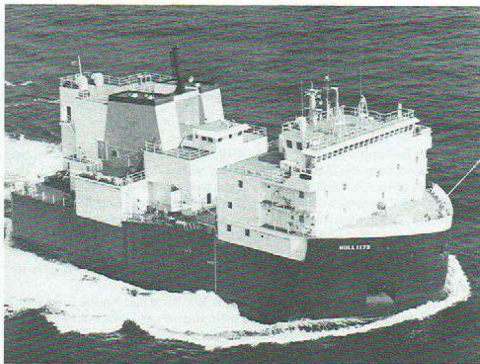
FIGURE 13. The bow and stern sections were constructed in Pascagoula, Mississippi by the Litton Ingalls Shipyard and were joined to make a ship capable of sailing from the Gulf along the Atlantic Coast and into the St. Lawrence Seaway to be joined with the mid-body at Erie, Pennsylvania.
