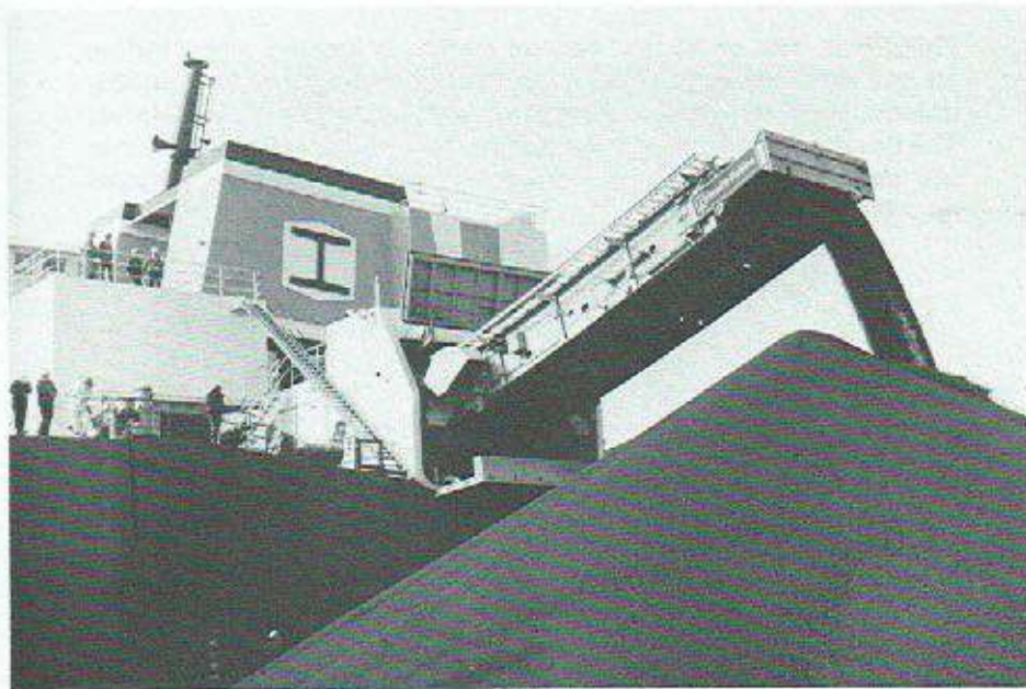
FIGURE 8. Pictured above is the unloading of iron ore pellets during testing at Erie, Pa. The unloading boom projects from the stern section of the ship and is capable of complete withdrawal within the sides of the ship. The unloading system on the vessel is designed for controlled output tonnage of a maximum 20,000 L.T./Hr. either into a hopper or to a dock surface.
