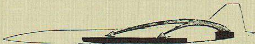
Figure 7: Concorde's Special Fuel Transfer System Used to Control the Aerodynamic Trim Change that Occurs During Transonic Acceleration and Deceleration.
