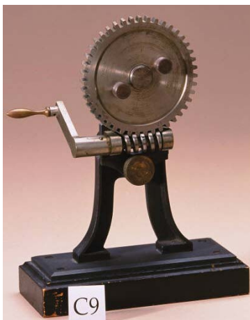
Reuleaux's version of the "endless screw."
