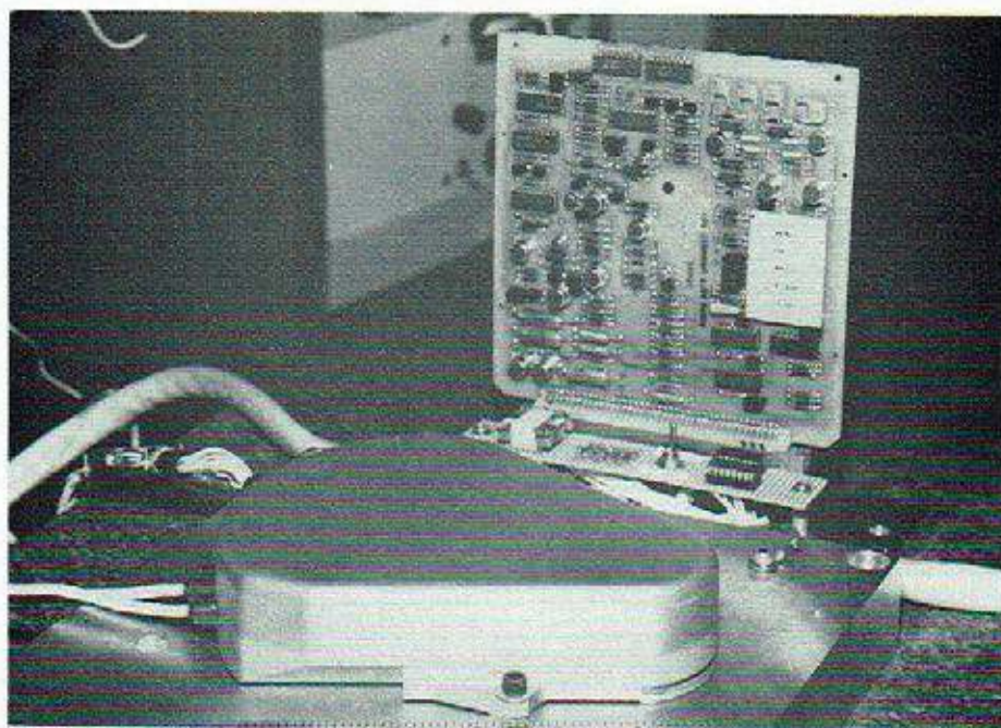
Figure 12. A picture of the production laser gyro and its remote, interchangeable electronics card.
