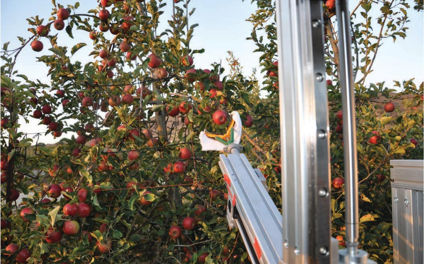
Attached to a slowly moving tractor, FFRobotics' arm needs only two degrees of freedom to pick most apples.
